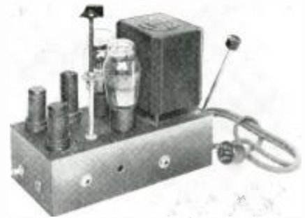
The amplifier chassis without its dust cover.
