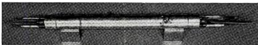
Two-stream amplifier is a modified traveling-wave tube with a bandpass of over 1,000 mc.
