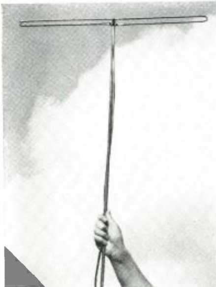
Fig. 4—Hand-held antenna used for testing.
