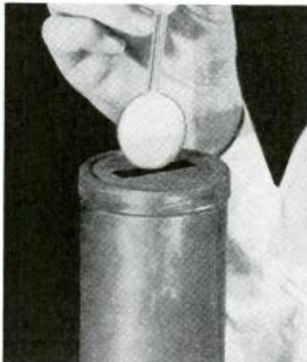
Fig. 7—Lifting electret from Faraday cage. tial curve predicted by E. P. Adams of Princeton University. The time required for the charges to reach maximum values is from 2 to 4 months. The growth of charge for one of the author's electrets is shown in Fig. 5. This graph
