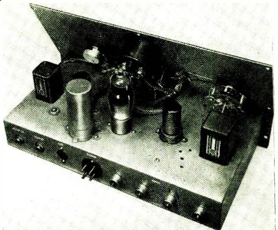
Photo shows chassis and panel pulled out of cabinet. Male power connector is used for safety.
