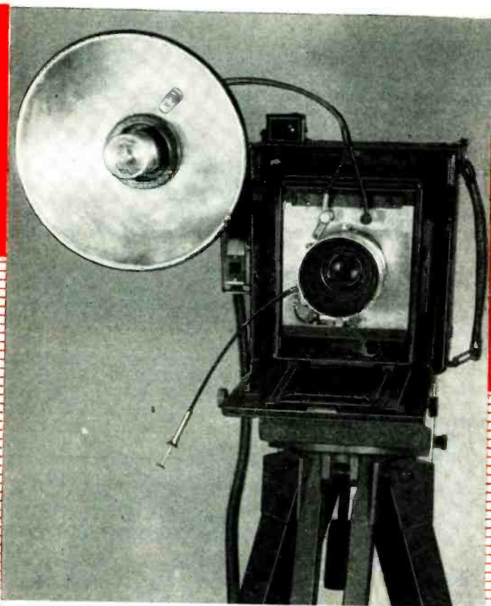
Synchronizing the flash gun is made easy by using a metal lens board.
