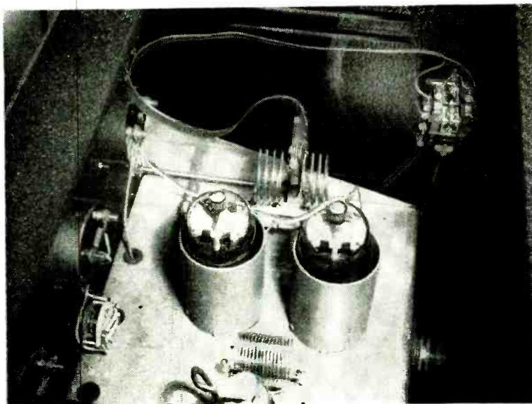
The two 813's and the plate coil are shown in the photo at the left. On the right the r.f. chassis is on the top, with the power supply-modulator below.
