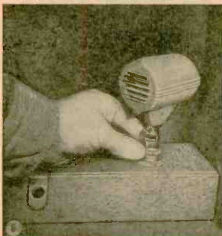
PHOTO 1.—In transporting, make sure the pickup arm is secured to its rest. In the model shown, tighten the thumbscrew provided to hold the arm in position. Other record players have similar means for protecting the pickup arm.
