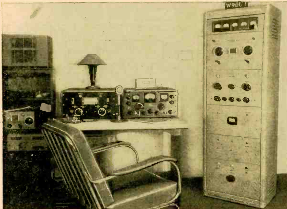
Operating position. Cabinet under lamp holds speech amplifier, monitor and remote switches.
