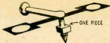
Fig. 5—Moving parts of tuned-ribbon pickup.
