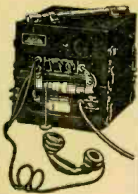
SCR-610 low power FM transceiver. Battery operation on 27mc to 38.9 mc. Less crystals $39.50
