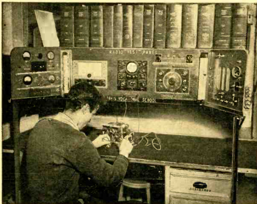
Test panel and service bench constructed by pupils of the Electric Shop, Dover (N.H.) High School. Power panel supplies 117 volts, 6 volts for farm and rural sets, and 2 volts.
