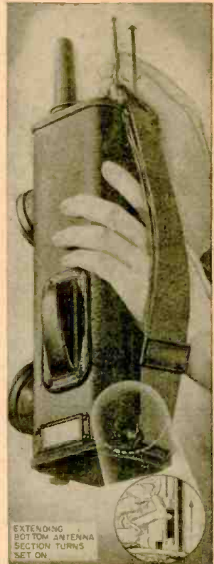
Antenna switch detail.
