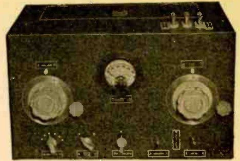
The Comparator. Connection to components being tested are made by posts at upper right.
