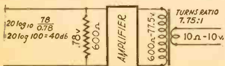
Fig. 2—Gain calculations for an amplifier.
