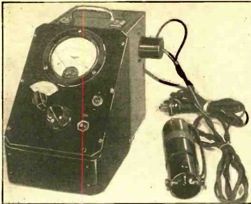
◀ View of completed V.-T. Voltmeter. The positive range switch is shown at left; zero-adjust, center knob; 110 V. power switch, lower-right, and negative to positive switch, upper-right. The prod tube shown at right connects by cable to the instrument through a plug-and-jack at the side of the case.
