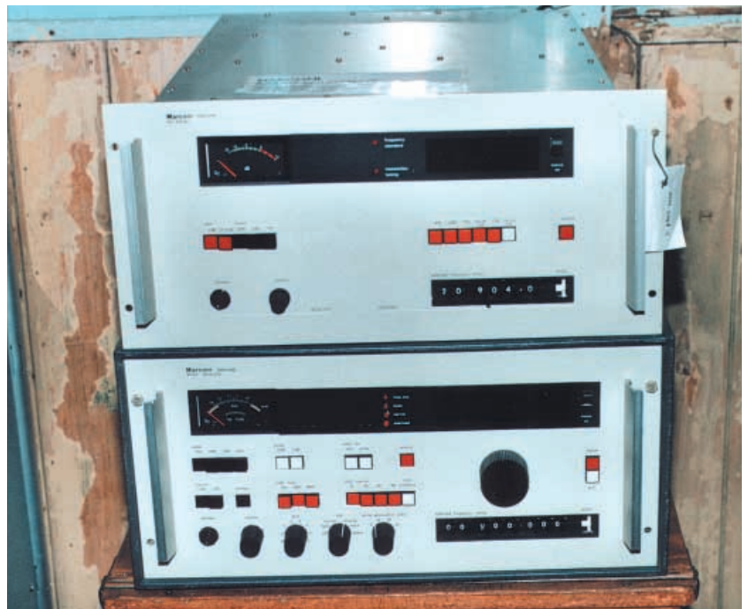
Two Marconi items from the 1980s, at the top is the H1540 driver and below is the H2540 VLF to HF receiver. The H2540 has come a long way since the CR100!
