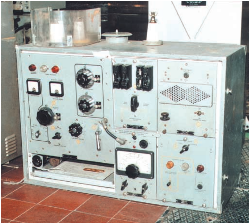
A ship's reserve receiver, transmitter and power supply, normally used when the main equipment has failed
