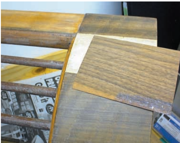
A section of the original veneer was removed and a new piece cut to replace it
