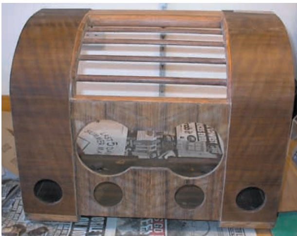
The cabinet ready to be refinished with toner spray, lacquer and wax
