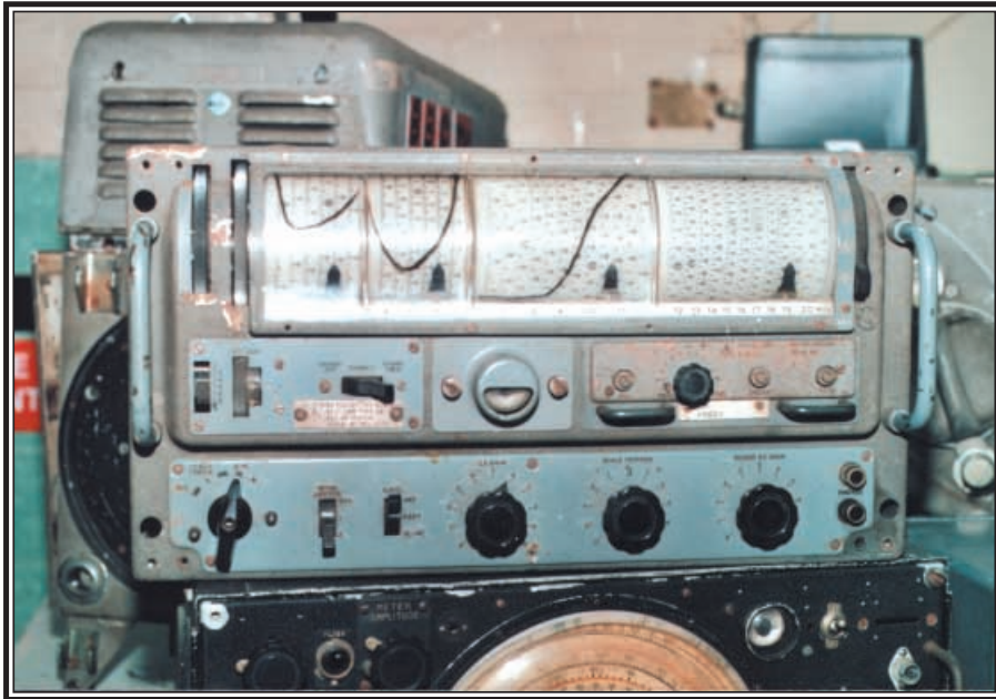
The wartime 1475 used by the RAF, sitting on top of another classic, the 1155 receiver
