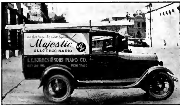
This is an ideal type of truck for radio service work. Note the ladder for making antenna installations.
