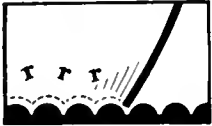
This is the action of the usual wire wound control after it has been in use for some time... like dragging a stick over a cobblesone pavement.
