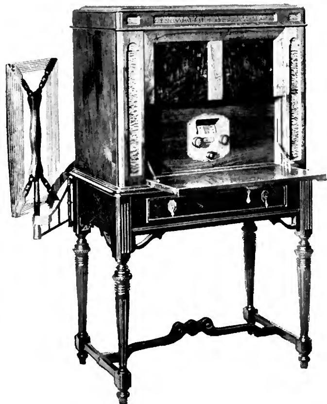
THE FADA 7 It is optional whether loop or antenna is used with this receiver, which has four stages of r. f. An improvement in the detector circuit reduces the possibilities of overloading. This seven-tube receiver sells for $185.00
