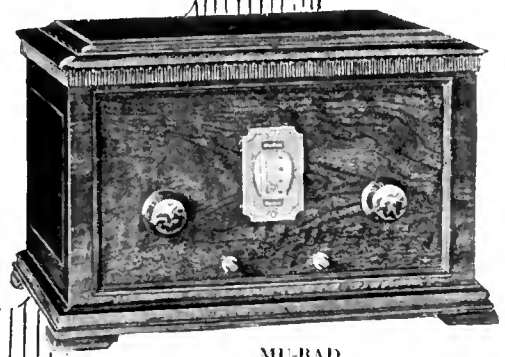
MU-RAD Two r. f. stages, detector, and three audio stages are included in this receiver. The audio stages, all of the double-impedance form, give uniform response between 30 and 5000 cycles, according to the manufacturers. Single-control tuning is featured. Price $98.00. In a console, equipped for complete a. c. operation, the receiver sells for $265
