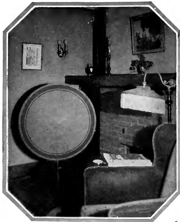
A THREE-FOOT CONE It is a fairly simple matter for the fan interested to make himself a three-foot cone, and obtain superior reproduction of music. The one illustrated to the left is described by the author and makes use of a Western Electric 540-AW unit
