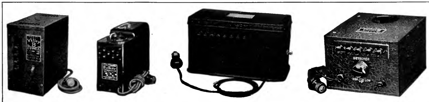
NEW UNITS FOR SUPPLYING B POWER
