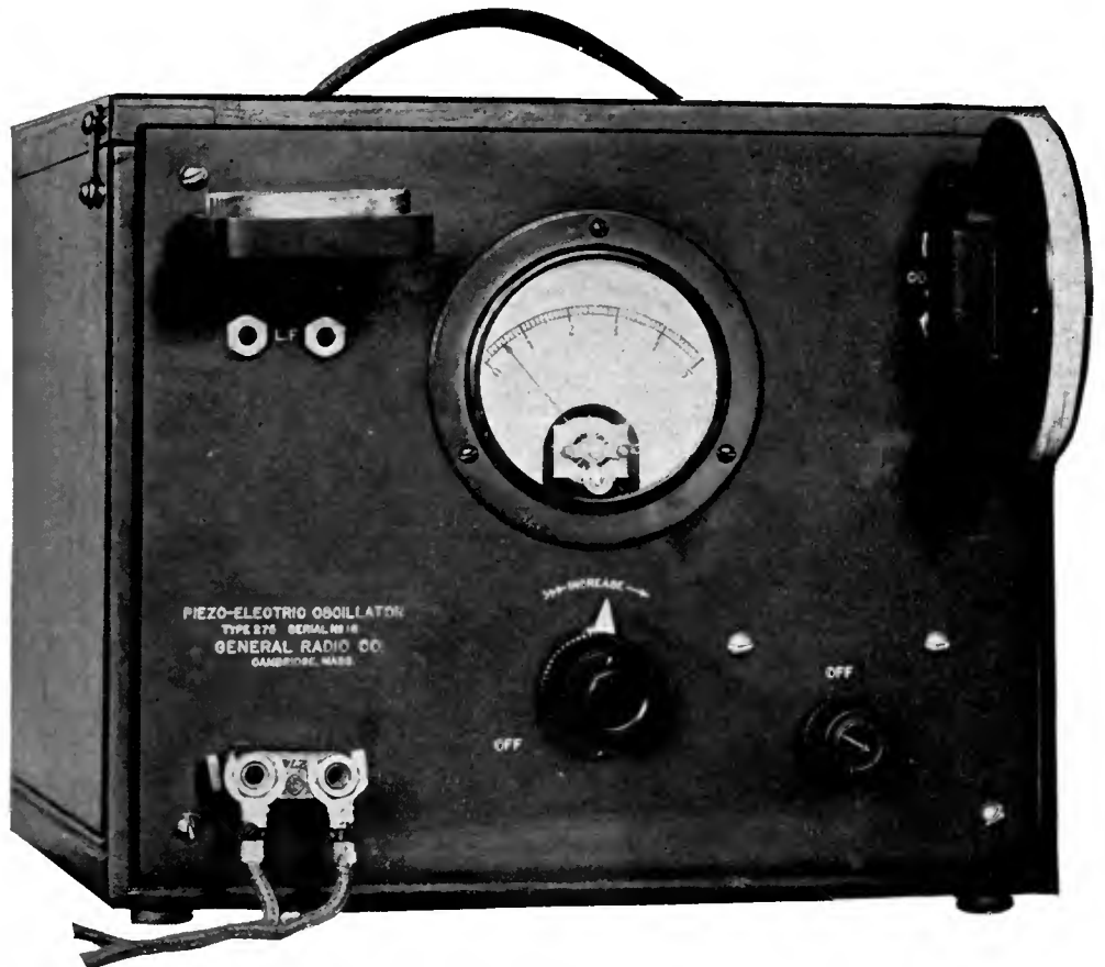
One scheme of circuit which will oscillate at the frequency of the crystal. Apparatus wired to give crystal-controlled oscillations is collectively called a Crystal Oscillator
