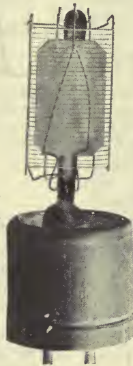
The filament, grid, and plate are seen here in their relative positions. The glass bulb has been broken away
