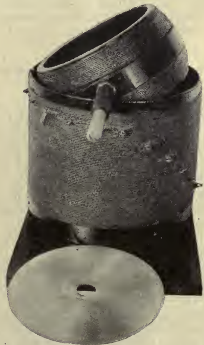
A SUITABLE VARIOCOUPLER For broadcasting or amateur reception, with its metal shield which reduces body capacity effects
