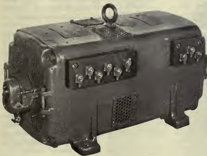
A 2-KW 500-CYCLE MOTOR-GENERATOR
