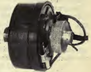
FIG. 6 The loud-speaking unit of a device which uses an adjustable magnet system
