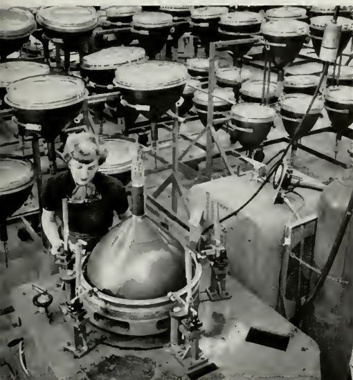
Welding a 19-inch tricolor tube at the Lancaster, Pa., RCA plant, where tube is in pilot production.
