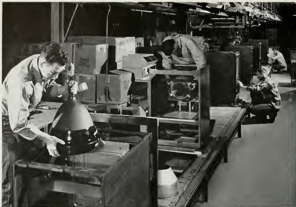
RCA tricolor tubes are installed in the first commercial production sets at Bloomington, Ind., RCA plant.
