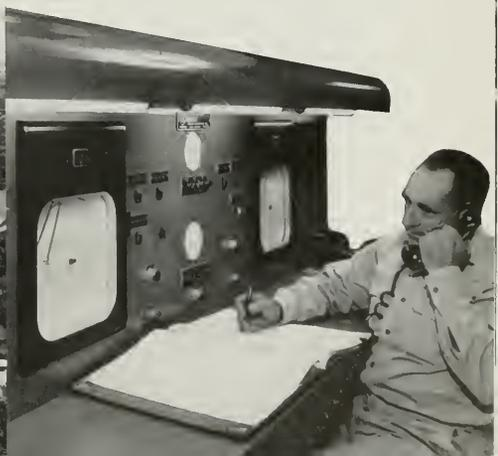
units, as well as handling telemetering and load control data. It is designed to handle 24 simultaneous voice conversations between any two points on the circuit. By clearing just one of the voice channels, as many as 18 simultaneous telemetering or load control functions may be added.
