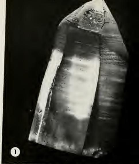
**1**—Specimen of Brazilian quartz from which come the crystal wafers that are used in the operation of millions of radio transmitters and receivers.
