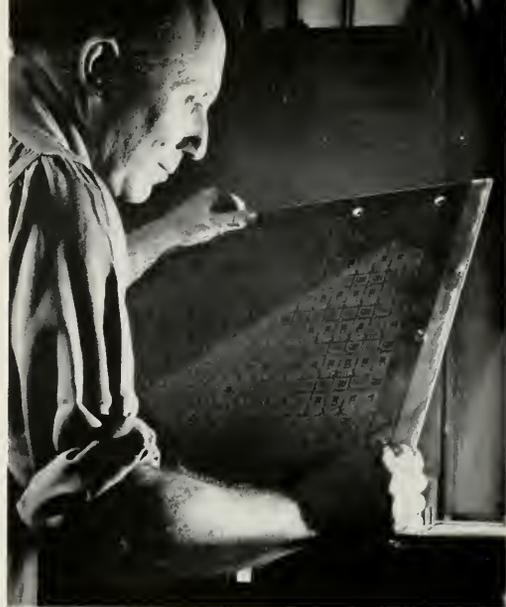
This glass negative will be used to produce an unlimited number of accurate replicas in an automatic photo-printing machine.
