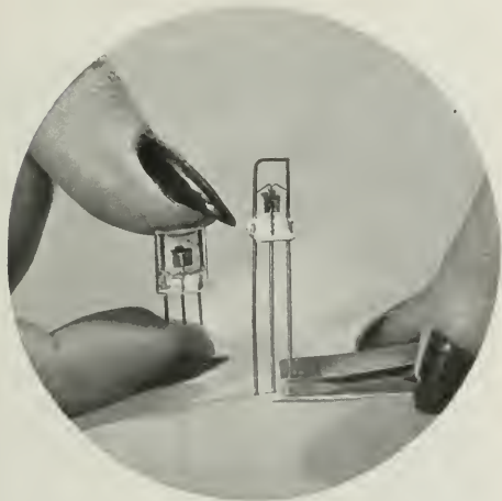
Point-contact type transistors before and after embedment in plastic housing.
