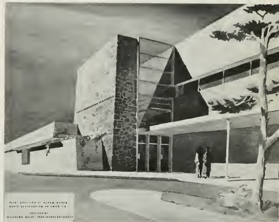
Architect's drawing of new facade to be constructed on the Bloomington, Ill., plant of RCA Victor Division. Production lines will occupy the first floor; offices above.
