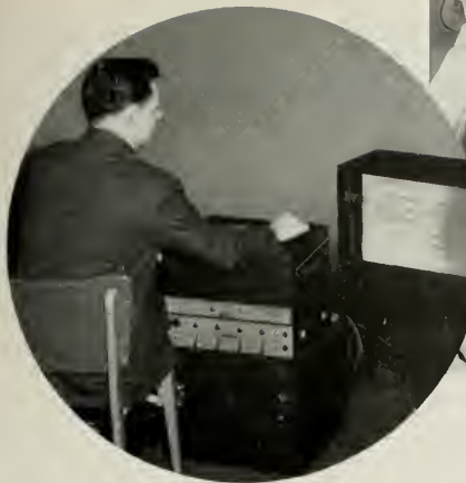
A Teleprompter user, reading his speech as it unrolls before him, is able to make his delivery sound extemporaneous. At left: An operator in the wings, working from an identical typewritten version of the text, adjusts the speed of the Teleprompter to the vocal speed of the speaker.
