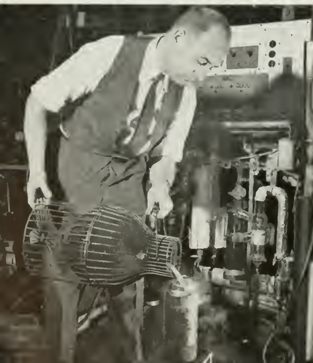
LIQUID AIR, TEMPERATURE 313 DEGREES BELOW ZERO, FAHRENHEIT, IS USED BY J. BURNETT TO IMPROVE THE VACUUM IN A TUBE WHEN IT IS COMPLETED. BELOW, H. A. FINKE TAKES PERFORMANCE DATA ON A BERESEARCH TUBE AS IT IS PUT THROUGH ITS PACES IN AN ELABORATE SERIES OF ELECTRICAL TESTS.
