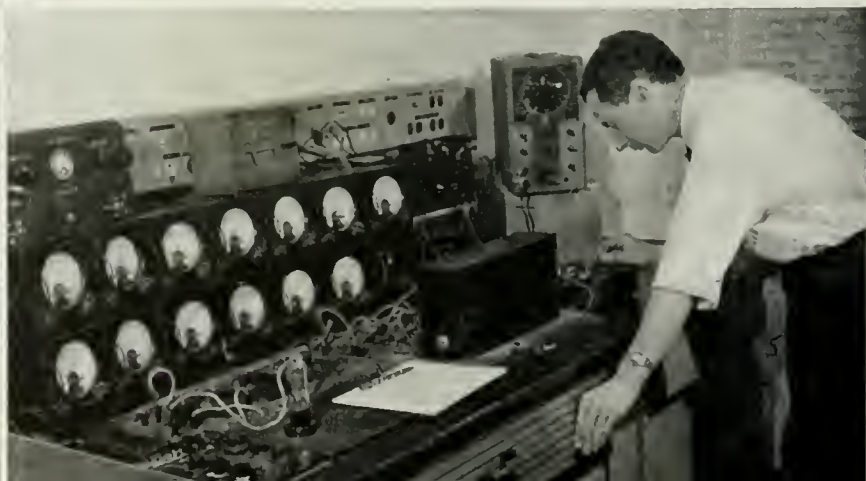
LIQUID AIR, TEMPERATURE 313 DEGREES BELOW ZERO, FAHRENHEIT, IS USED BY J. BURNETT TO IMPROVE THE VACUUM IN A TUBE WHEN IT IS COMPLETED. BELOW, H. A. FINKE TAKES PERFORMANCE DATA ON A BERESEARCH TUBE AS IT IS PUT THROUGH ITS PACES IN AN ELABORATE SERIES OF ELECTRICAL TESTS.
