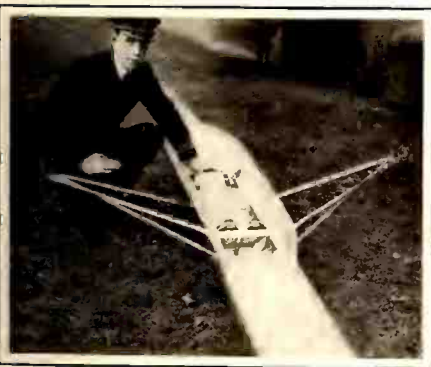
A single scull shell of duraluminum, a light but extremely durable alloy, has just been completed at the Philadelphia Naval Aircraft factory for the Annapolis Naval Academy. The shell weighs half as much as the cedar craft of the same type and size. It was built under the direction of Walter Hoover, noted single sculls oarsman. If the shell proves satisfactory, the Naval Academy expects to have an eight-oared shell constructed of the material. It is 26 feet long and weighs only 26 pounds. Photo shows Lieut. Calvin Bolste, shop superintendent, inspecting the duraluminum shell.
