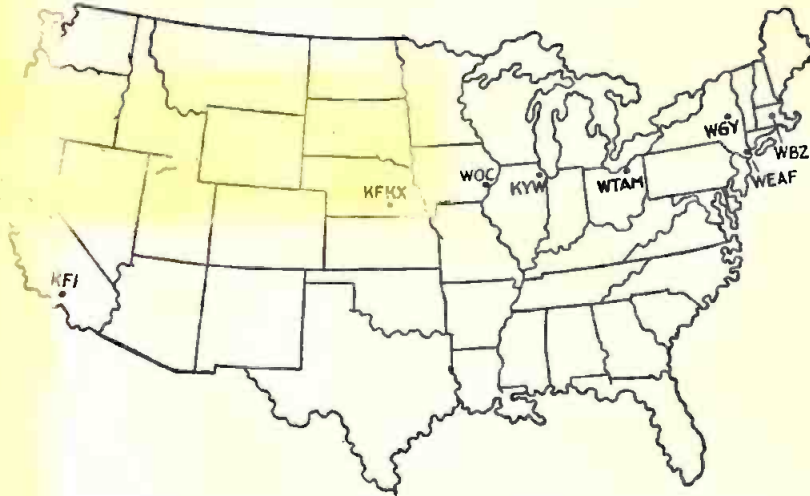
The map showing the first distribution of super-power broadcast stations throughout the country. Note that no two are close enough to seriously interfere with each other. KGO and KFI may prove exceptions, for they are not very far apart, but Government officials assure radio fans the air will not be congested by the strong stations.
