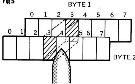
"Each pixel is controlled by 2 bits - one from each byte"
