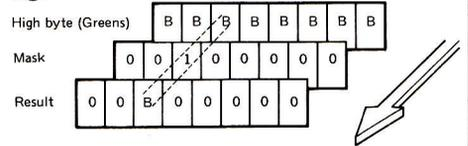
shown in fig. 7 allowing the result through from that bit number only. This is done by using the AND function.
