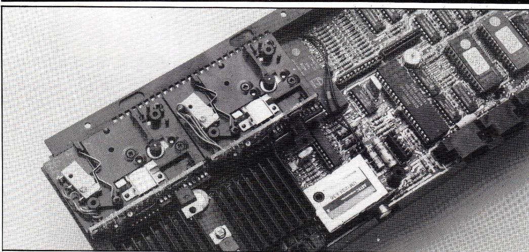
The much-maligned microdrive mechanism revealed for all to see.
