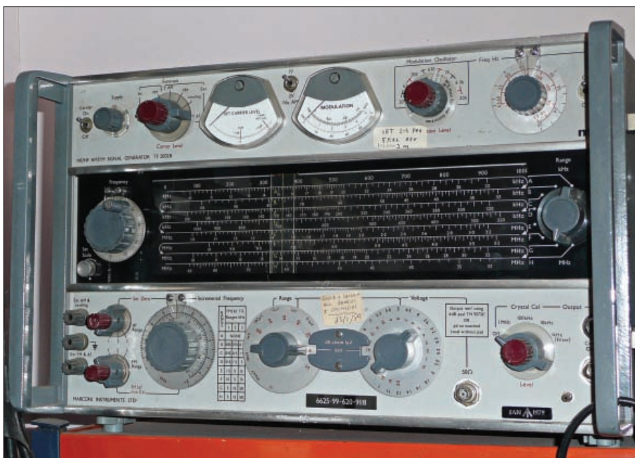
Fig. 1: Harry's trusty TF2002B covers down to the upper audio band as well as its r.f. option.
