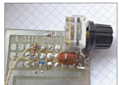
Fig. 3: Regular PW author Roger Laphorne G3XBM's circuit uses a toroidal core.
