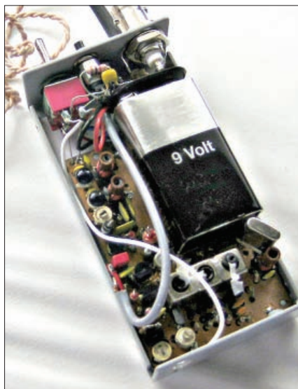
Internal view of the Fredbox clearly demonstrating how much space the battery takes up.
