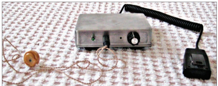
Roger's Fred Sixbox ready for use on 50MHz. The earphone and microphone provides an idea of the physical size of the rig.
