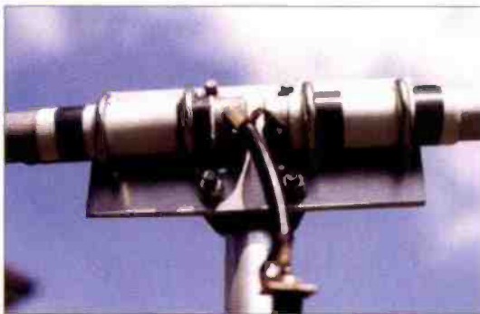
Fig. 6: Driven element centre insulator section. The elements are insulated from the plate and the U-bolts with thick PVC insulation, which is taped to the elements before fixing in place.
