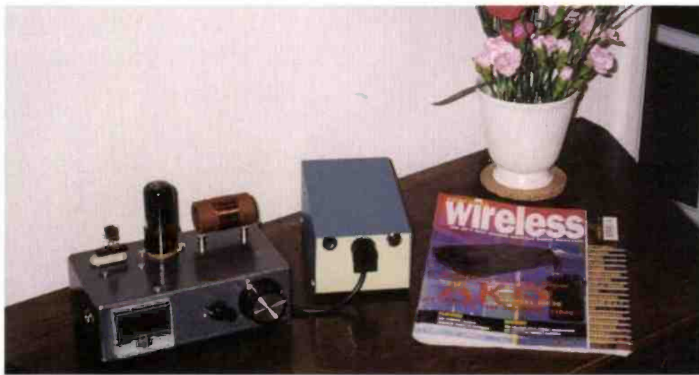
Fig. 3: Photograph showing the (very neat-looking) 6V6GT one-valved transmitter, from an article incorporating a classic design and published in the December 1997 PW (see text).
