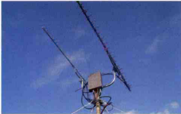
Fig. 4: 1.3GHz Yagi and 2.3GHz Quad Loop Yagi.
