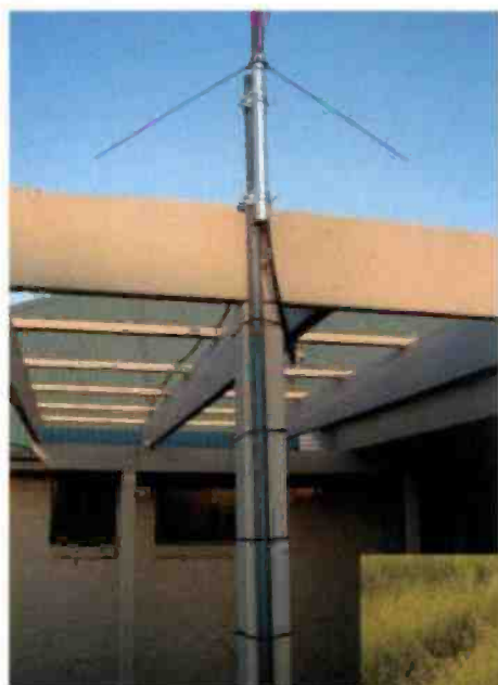
Fig. 1: Chris VK3CE's antenna which was very quickly set up for the 'Remembrance Day Contest' - with nothing more than a few plastic cable ties holding it vertical!
