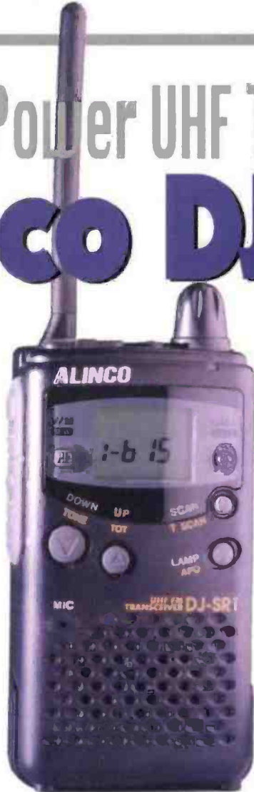
The Alinco DJ-SR1 PMR-446 licence free, low power, u.h.f. transceiver.
