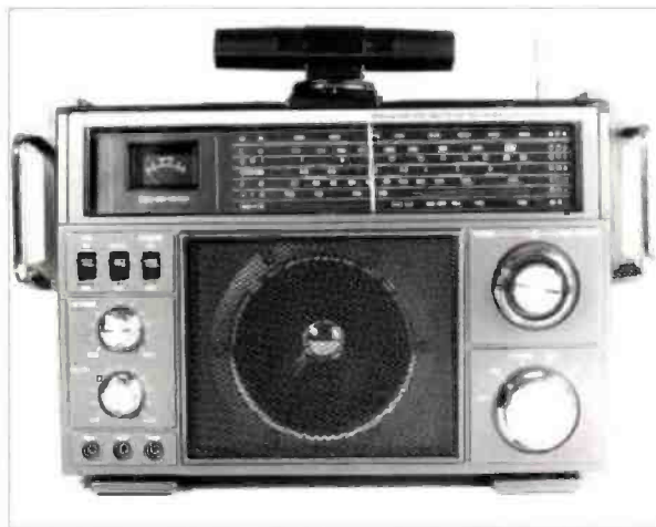
Fig. 2: There are many receivers - such as this 'Steepletone' - in use. The advantages with the larger dial means that 'fine' tuning is easier because of the larger scale (see text).
