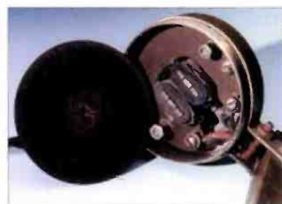
Fig. 5: A truly 'vintage' earphone, illustrated with the 'Stalloy' metal diaphragm slid away. (They must never be pulled away from the magnet to expose the high impedance (approximately 2kΩ) windings around the permanent magnets).
