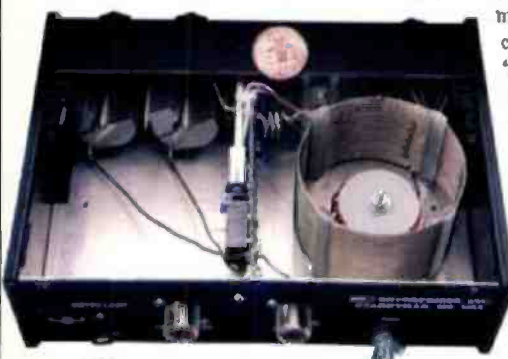
Fig. 1: Inside the MFJ-45E showing the substantial inductor. An idea of the size of the unit is provided by the two pence coin above the front panel. Meter illumination is provided by the 'Meter Lamp' socket on the left of the rear panel.
