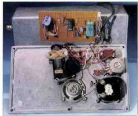
Fig. 3: An inside view of the unit showing method of construction using Veroboard (see text).
