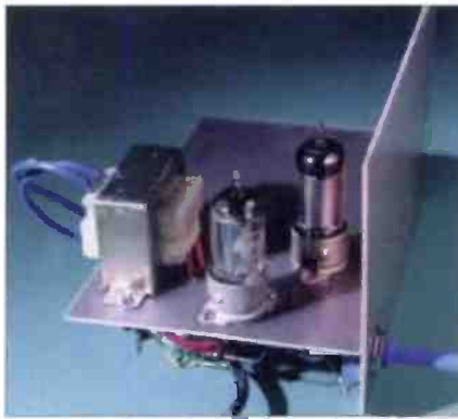
Fig. 8: The prototype audio amplifier from above. Space has been left at the other side of the unit to include a receiver at a later date.
