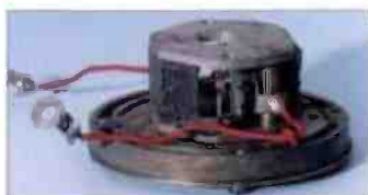
Fig. 6: Close up view showing the mechanism inside a 'balanced armature' earpiece. Extremely versatile and sensitive, this form of earpiece insert is extremely robust and many examples made between 1939-45 are still in service.
