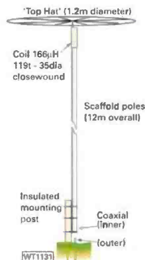
Fig. 5: A round capacity, or 'Top hat' loading element on a free-standing vertical suitable for use on 1.8MHz (see text).
