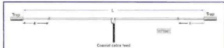
Fig. 3: Each element is treated to a first adjustment individually and without the outer element fitted.
