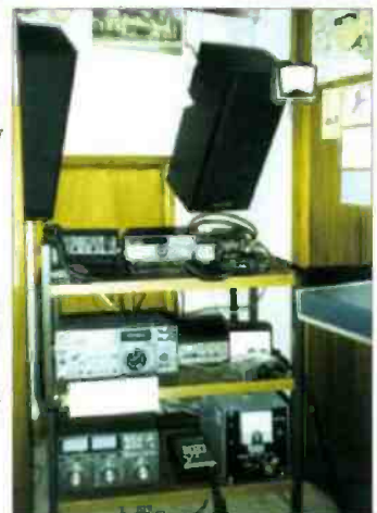
Fig. 4: Part of G4VfV's shack, showing the pair of hi-fi loudspeakers (not in stereo mode!) individually connected to 144MHz and h.f. transceivers.
