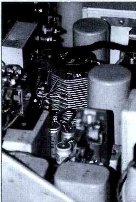
Fig. 4: Close-up view of the p. a. stage coil with associated tappings in the 11 set. The two screening cans visible shield valves (see text).
