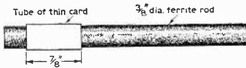
Fig. 4a: Stage 1 of construction of long wave coil.
