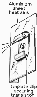
Fig. 4: The transistor heat sink for Tr6 and Tr7.
