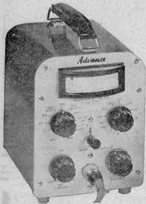
This instrument from Advance Components Ltd. checks transistors in circuit.
