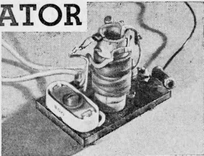
A view of the crystal receiver used for testing.
