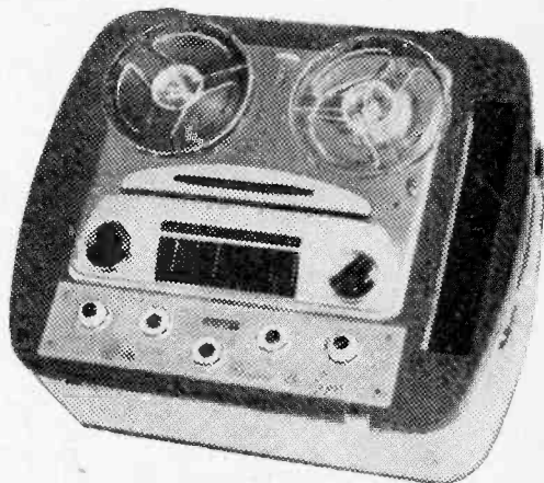
The new "Sound Master" tape recorder is a 3-speed, 4-track model.
