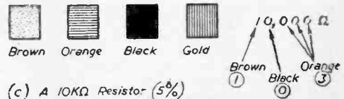
Fig. 4.—Reading the resistor colour code.
