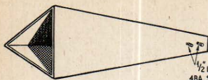
Fig. 2a. Half of the "bow tie" element for the loft aerial. The soldered join is along the back edge or "apex".
