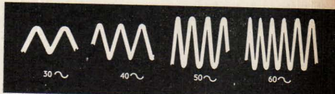
Fig. 4. Waveform of the output of an 8in unit in a 1 cu ft enclosure with slotted back and an input of 1 watt
