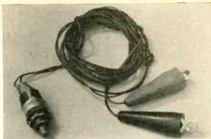
Simple gadget for turning over engine consists of two clip leads connected to normally-open push-button switch. Leads are connected to starter control terminals of starter solenoid.
