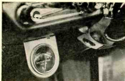
This illuminated voltmeter is one of several types for use in cars. Panel meters will also serve; in some cars, they can be mounted in dash. Meter above is sold by Lafayette Radio.
