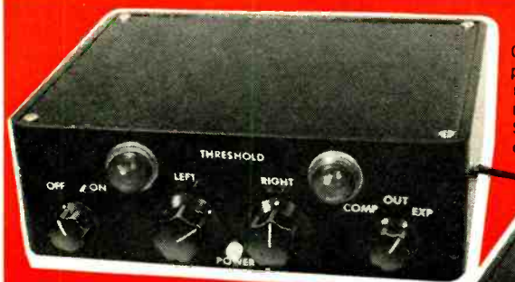
Controls on front of unit (photo above) are threshold controls which determine the level at which expansion or compression takes place. Panel lamps I1 and I2 glow in proportion to the voltage of the audio tapped from speakers; switches control power, function.
