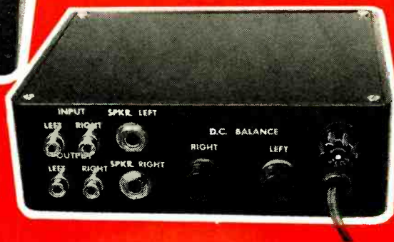
Controls on front of unit (photo above) are threshold controls which determine the level at which expansion or compression takes place. Panel lamps I1 and I2 glow in proportion to the voltage of the audio tapped from speakers; switches control power, function.
