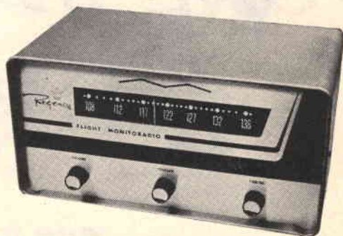
Typical receiver for monitoring aviation radio signals as a hobby is the Regency "Flight Monitoradio."
