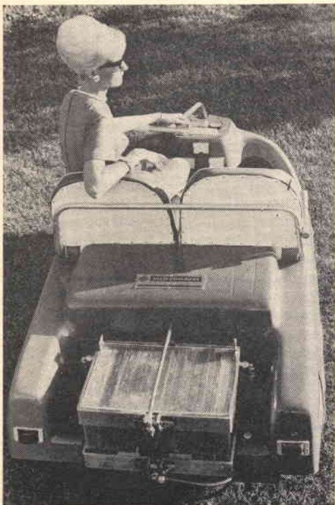
This fuel-cell-driven golf cart made by Allis-Chalmers shows the feasibility of putting fuel cells to work powering vehicles. A fuel-cell-operated farm tractor was demonstrated by firm as early as 1959.
