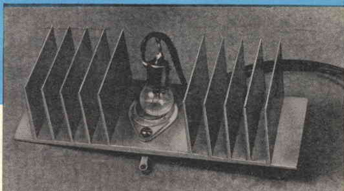
Assembled heat sink is shown below, before encapsulation and painting.
