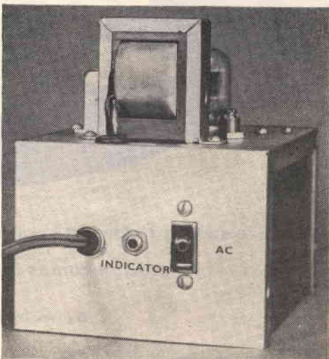
Indicator lamp jack is connected to miniature plug so lamp can be mounted at tuner or amplifier panel.
