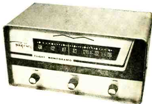
Typical receiver for monitoring aviation radio signals as a hobby is the Regency "Flight Monitoradio."
