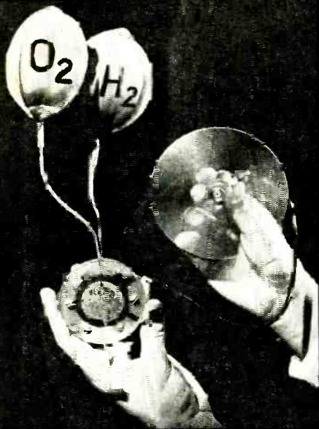
A hydrogen-oxygen fuel cell circa 1959 shows immense progress that has been made in a few years. Object at right of S.E. cell is a motor with a propeller.
