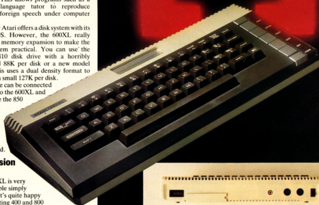
Above: The 600XL has outputs for TV and monitor, a standard Atari peripheral port and a new Parallel bus
