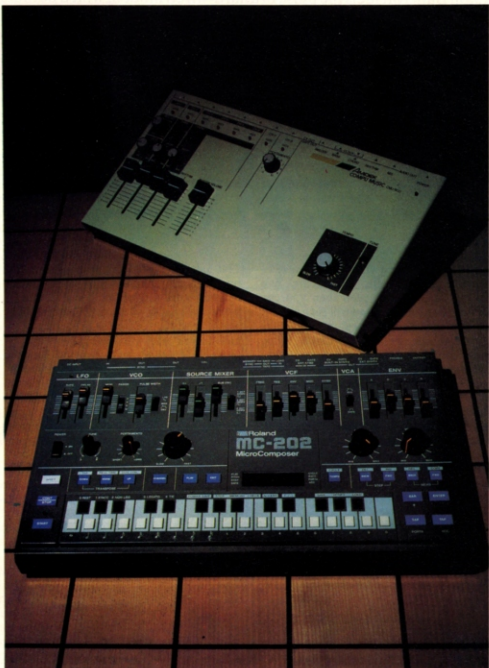
Roland's hardware: Compu-Music (top) gets its musical instructions from Apple software; the Micro-Composer stand-alone musical computer (bottom).
