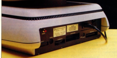
Reset button, RS232, video, cassette (would you believe!), cartridge, Earth, audio and IEEE 488 — connections in that order.
