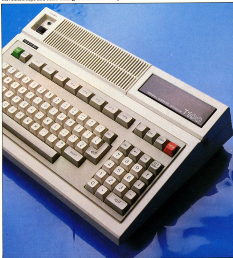
Top right is a hinged panel which opens to reveal sockets for the ROM and RAM packs. The cursor movement keys and some editing functions are neatly collected below it.
