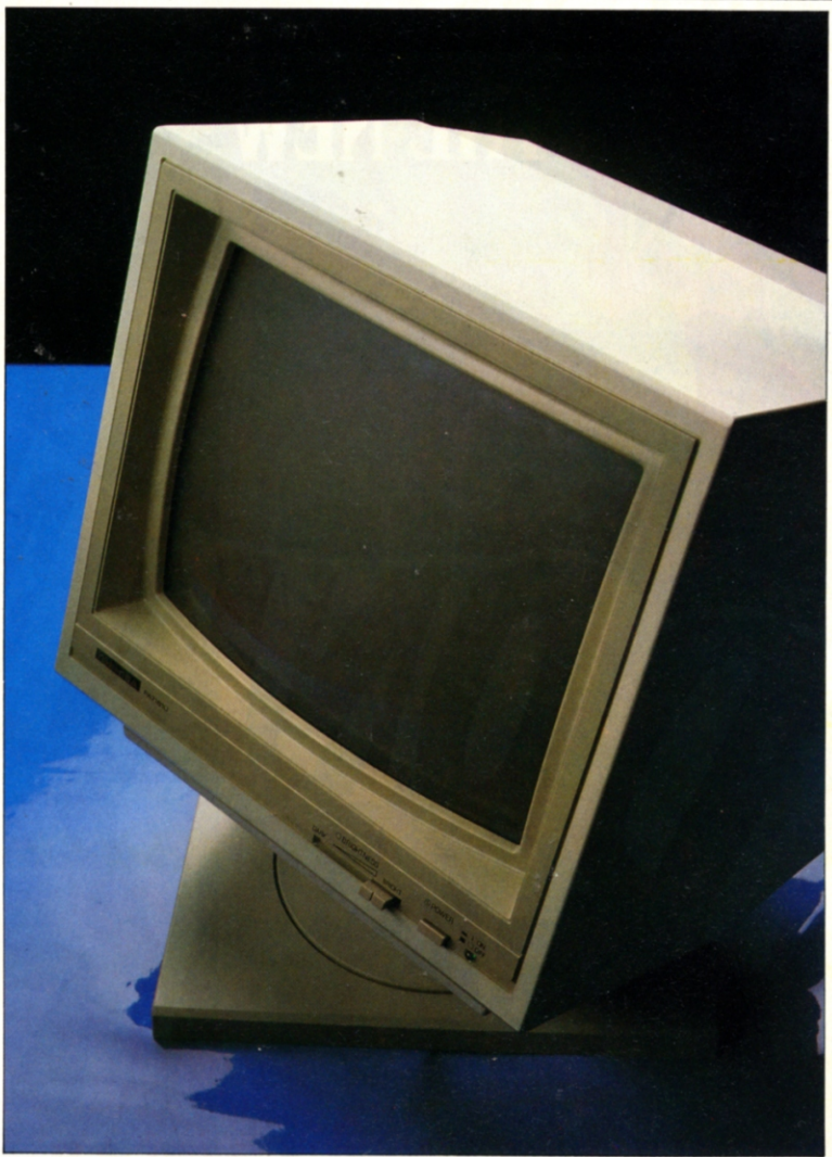
The VDU tilts and swivels to prevent cricks in the user's neck.
