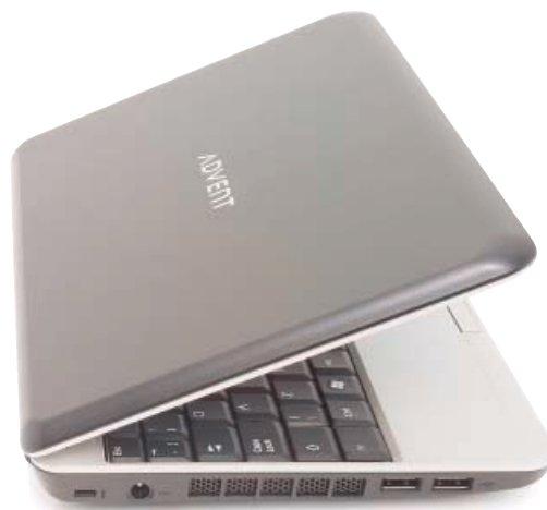
The Advent 4211 sports Intel's new Atom N270 processor, making for an exceptionally quiet-running machine
