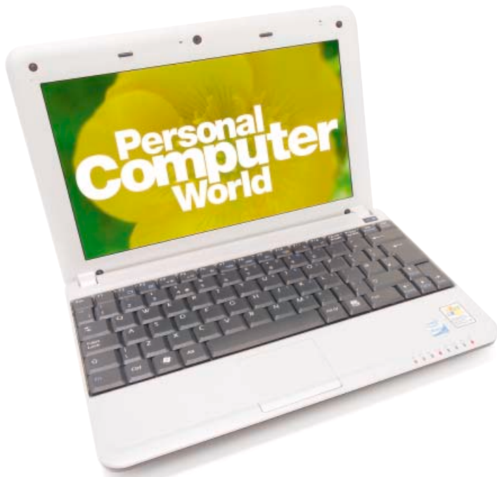
The Advent 4211 sports Intel's new Atom N270 processor, making for an exceptionally quiet-running machine
