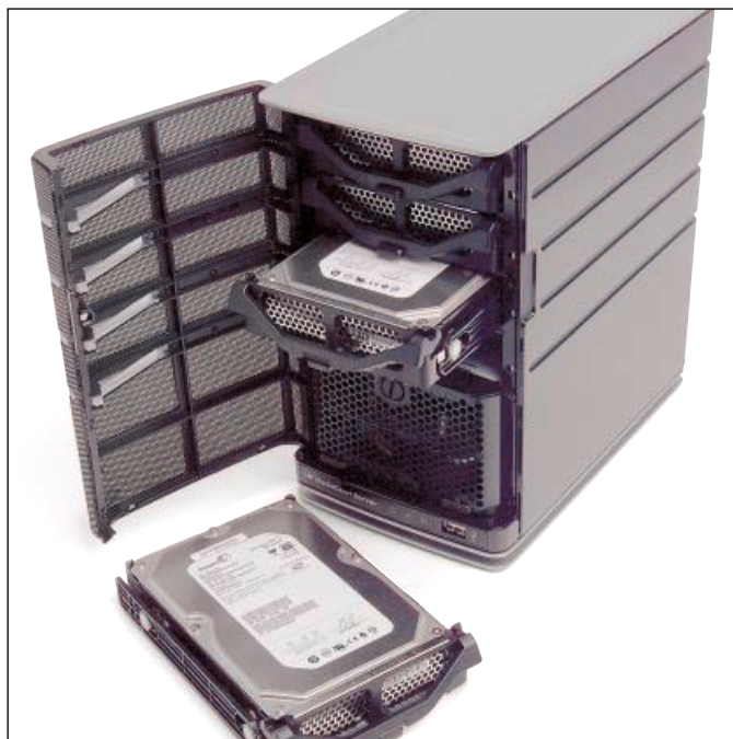
The Mediasmart has four horizontally arranged SATA hard drive caddies for storage, with lights alongside each drive to indicate which caddies are occupied. The caddies are easy to remove and a grilled door allows for excellent ventilation.
