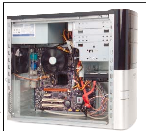
There's plenty of room inside the case, including a spare internal bay for fitting an extra hard disk
