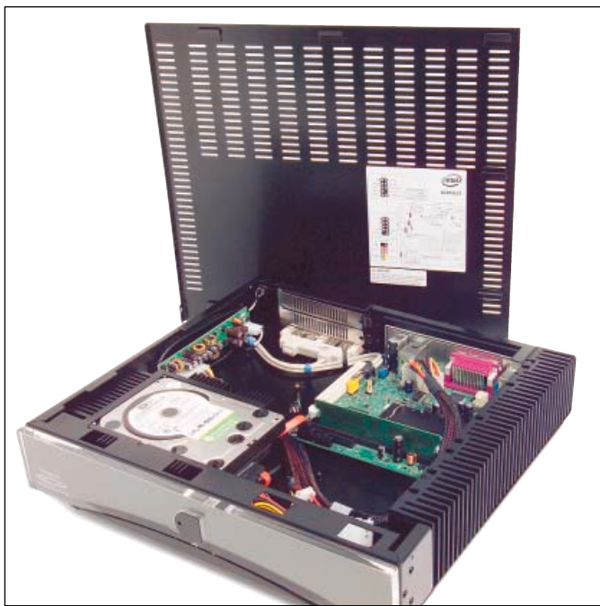
Opening up the T2-WHS-A3 reveals an awesome array of heatsinks and no fans. Three PCI-sized backplates (one was occupied by USB ports on our model) means you can add more connectivity or other hardware.
