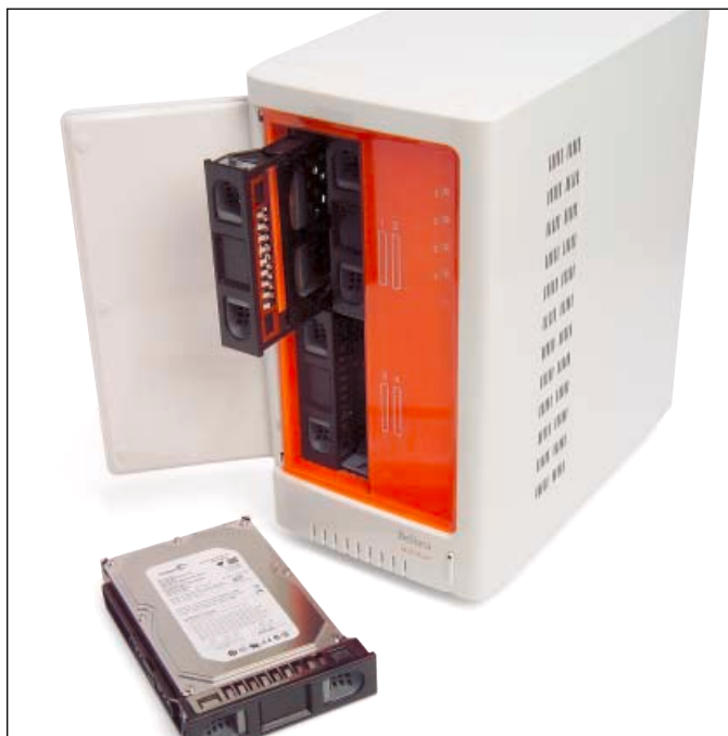
The O.center uses four vertically arranged SATA hard drive caddies for storage, protected by a swing-out door. The caddies are more stubborn to remove and replace than on the Mediasmart, but they are tougher.
