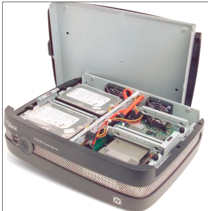
The side panel must be removed for access to the Scaleo's hard drives, revealing two large system fans, which are noisy when starting up. There's space for four drives, in paired scaffolding that can be lifted out of the server.
