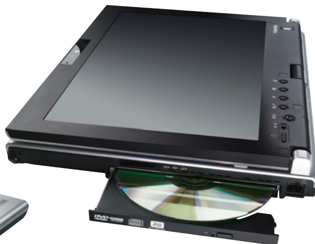
There are some interesting features on the M700-110, including two latches which lock the screen in position to prevent it from twisting during use
