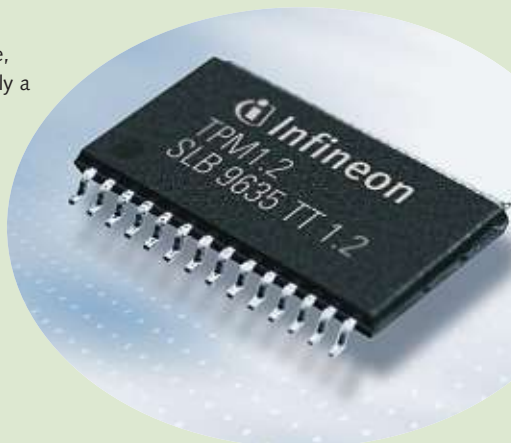
Hot topic: the TPM chip makes it possible to digitally sign content
