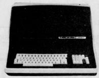
NOW WITH CP/M 2.2, & NOW WITH CP/M 2.2, & INCREASED DISC STORAGE. TWIN 280-A 1MHZ \* 2 DISC DRIVES, DUAL DENSITY 320 K QUAD DENSITY 700 K STORAGE 64 K RAM \* HIGH RESOLUTION 12 INCH CRT. 80 x 24 LINES UPPER/LOWER CASE \* 2 RS-232 PEINTEP PAPES - 2 CPM 23 PRINTER PORTS \* CPM 2.2 OPERATING SYSTEM \* MBASIC, COBOL, FORTRAN, PASCAL, WORD PROCESSING & ACCOUNTS PACKAGES AVAILABLE DEALER ENQUIRIES INVITED
