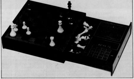
Sargon 2.5, showing the board, set (provided), storage space and, on the righthand side (from top to bottom): plug-in module, display, clip-on keyboard.
