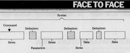
Figure 2: The Elements of a Free-format Message
