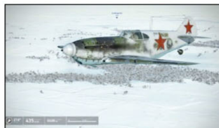
3. Note the exhaust flames – their colour can be used to determine if the mixture is set correctly.
