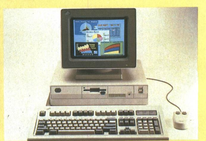
● While the rest of the PS/2 range features IBM's new MCA expansion bus, the Model 30 286 shown here has the standard AT-style bus. For a 286 it is pretty slow at 10MHz, and you pay nearly £1000 extra for the name.
