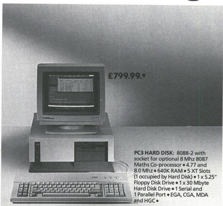
**PC3 HARD DISK:** 8088-2 with socket for optional 8 MHz 8087 Maths Co-processor • 4.77 and 8.0 MHz • 640K RAM • 5 XT Slots (1 occupied by Hard Disk) • 1 x 5.25" Floppy Disk Drive • 1 x 30 Mbyte Hard Disk Drive • 1 Serial and 1 Parallel Port • EGA, CGA, MDA and HGC •
